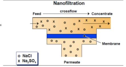
Figure 1. Principles of Nanofiltration
