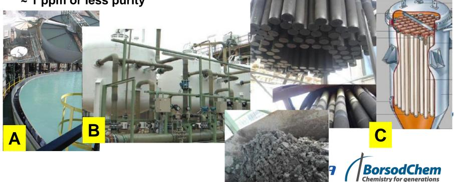
A. Ion exchange using a special chelating resin mixture to remove residual dissolved metal ions  $\rightarrow$  super pure brine Concentration, pH, resin regeneration mode are extremely important Regeneration: with high purity NaOH and hydrochloric acid (self-produced)
